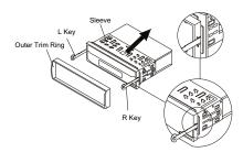
5. Mount the sleeve by inserting the sleeve into the opening of the dashboard and bend open the tabs located around the sleeve with a screwdriver. Not all tabs will be able to make contact, so examine which ones will be most effective. Bending open the appropriate tabs behind the dashboard to secure the sleeve in place.
